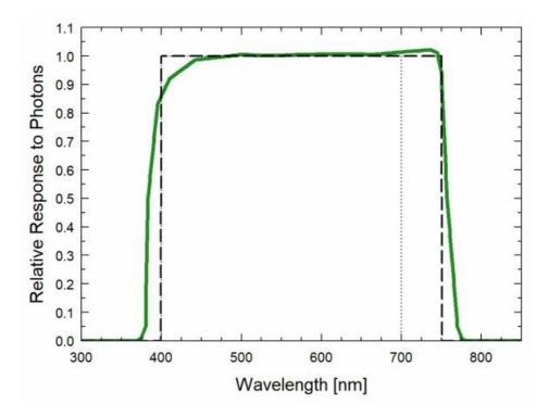
Mean spectral response measurements of four replicate Apogee SQ-600 series ePAR Sensors. Incremental spectral response measurements were made at 10 nm increments across a wavelength range of 370 to 800 nm in a monochromator with an attached electric light source. Measured spectral data from each quantum sensor were refined and normalized by comparing measured spectral response of the monochromator/electric light combination to measured spectral differences from a quantum sensor reference.
