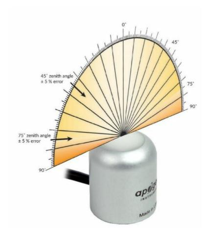
Directional, or cosine, response is defined as the measurement error at a specific angle of radiation incidence. Error for Apogee SQ-600 series ePAR Sensor is approximately  $\pm$  2 % and  $\pm$  5 % at solar zenith angles of 45° and 75°, respectively.
