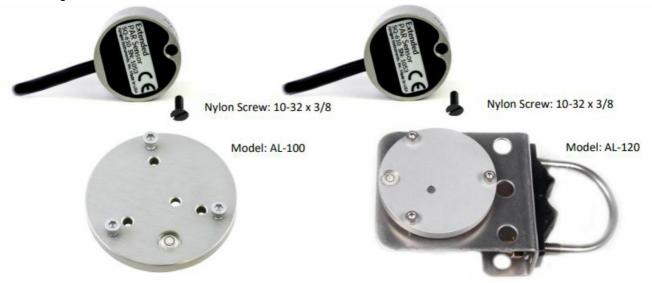
To minimize azimuth error, the sensor should be mounted with the cable pointing toward true north in the northern hemisphere or true south in the southern hemisphere. Azimuth error is typically less than 0.5 %, but it is easy to minimize by proper cable orientation.
