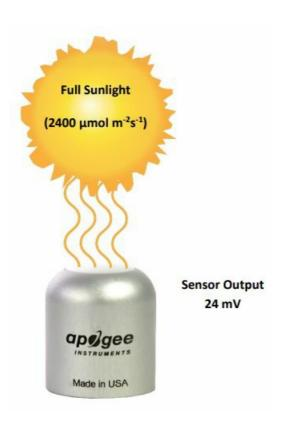
Example of photon flux density measurement with an Apogee model SQ-610 ePAR Sensor. Full sunlight yields a photon flux density on a horizontal plane of approximately 2400  $\mu$ mol m-2 s-1. This yields an output signal of 24 mV. This signal is converted to photon flux density by multiplying by the calibration factor of 100 mol m-2 s-1 / mV.
