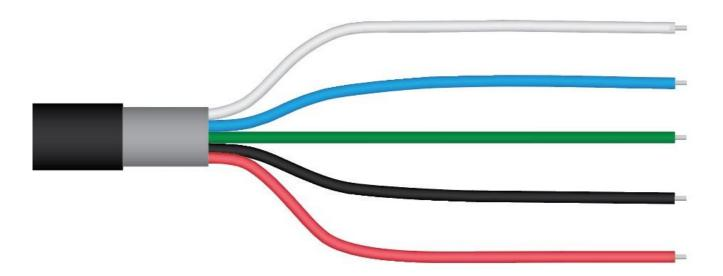
The Green wire should be connected to Ground to enable RS-485 communication, or it should be connected to 12 V power for RS-232 communication. Text for the White and Blue wires above refers to the port that the wires should be connected to.
