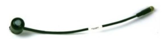
When sending sensors in for calibration, only send the short end of the cable and half the connector.
