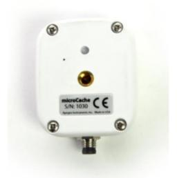
The sensor model number and serial number are located on the back of the  $\mu$ Cache unit. If you need the manufacturing date of your  $\mu$ Cache, please contact Apogee Instruments with the serial number of your  $\mu$ Cache.
