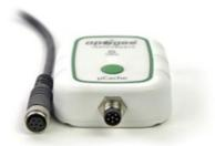
The  $\mu$ Cache has an M8 connector that is used to connect to an analog sensor.
