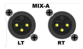
MIX-A and MIX-B LT and RT: Left and Right Mix-A and Mix-B stereo output connections
