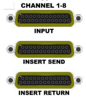
NOTE: Because 25-pin Dsub connectors are used for all I/O, there is no possibility for normalling the INSERT RETURN. So, if a channel INS switch is engaged and no signal connected to the INSERT RETURN, the audio on that channel will be interrupted.
