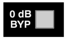
dB BYP (Bypass): Bypasses the channel level control and sets the channel levels to unity gain on all input channels when engaged
