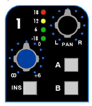
Input channels 1-16 are designed to accept any external balanced, line-level, low-impedance analog audio signal from the rear panel DB25 connectors and assign them to the Mix-A and/or Mix-B stereo buses. A balanced, line-level, low-impedance analog audio insert is provided via the INS switch and rear panel connectors.
