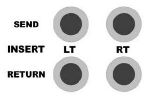
Mix LT - RT INSERT SEND: Stereo insert send connections for Mix-A and Mix-B
