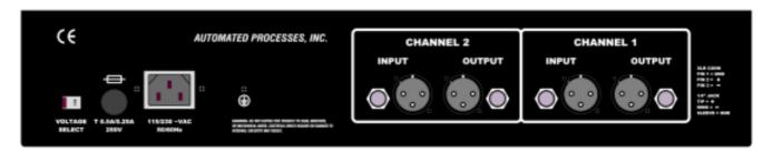
The inputs to the SR24 can be either the 3 pin XLR-type balanced connector or the 1/4" balanced (tip, ring, sleeve) jack. Note that if you were to connect to both connectors, the signal from the 1/4" jack takes priority. The input XLR connector is wired pin 2 hot (or +).
