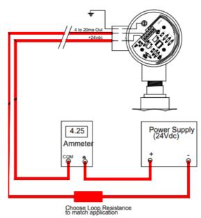
Step 1. Set DC power supply voltage at 24VDC.
