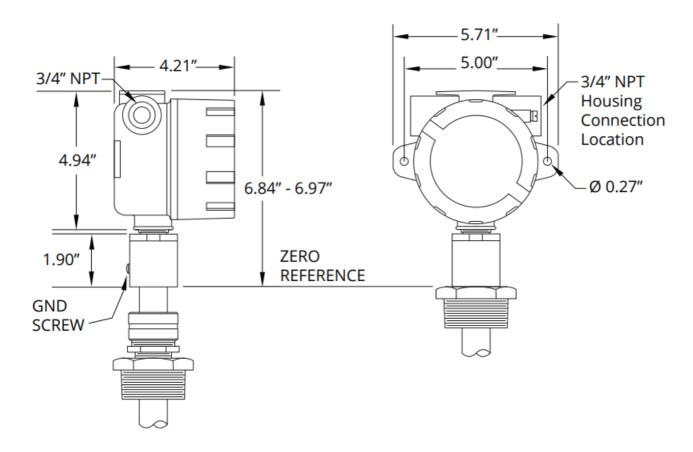
**DANGER:** OPEN CIRCUIT BEFORE REMOVING COVER or KEEP COVER TIGHT WHILE CIRCUITS ARE ALIVE;
