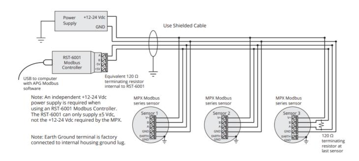
**IMPORTANT:** For EMI protection on an MPX-T4 or MPX-T5, either connect the grounding screw (see section 4) to an earth ground, or ensure that tank mounting of the MPX is grounded.
