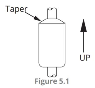
**IMPORTANT:** Floats must be oriented properly on the stem, or sensor readings will be inaccurate and unreliable. Untapered floats will have a sticker or "N" indicating the top of the float. Remove sticker prior to use.
