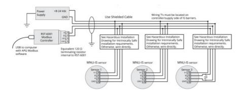
**Note**: An independent +8-24 Vdc power supply is required when using an RST-6001 Modbus Controller. The RST-6001 can only supply ±5 Vdc, not the +8-24 Vdc required by the MNU-IS.
