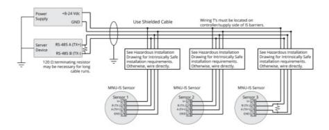
**Note:** When connecting MNU-IS sensors to your system, reversing A and B connections may be necessary if sensors do not communicate with Modbus Server device.
