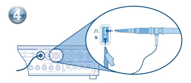
Connect the probe hook tip to the tab and the ground lead to the tab.
