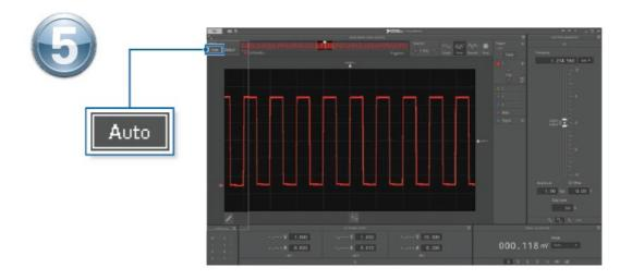
Click Auto to configure the oscilloscope for visualizing the 5 V, 1 kHz square wave generated the probe compensation tabs.
