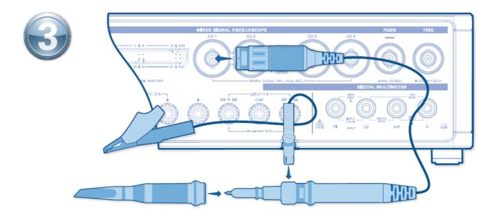
Attach the hook tip and ground lead to the oscilloscope probe. Then connect the probe to CH 1.
