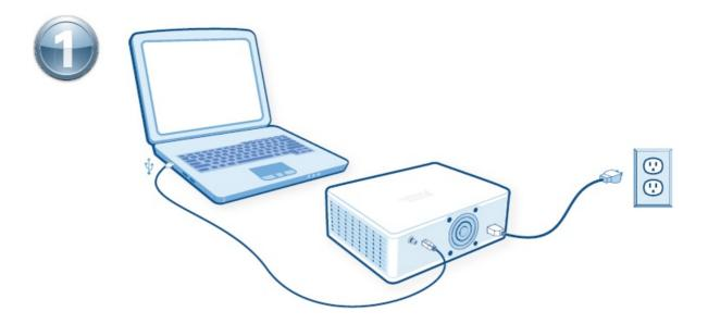
Connect the power cable. Then connect the Virtual Bench to a USB port on your computer.
