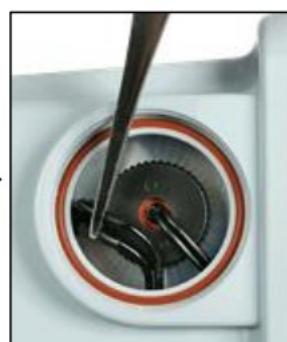
Use a tweezer to plug wire into the gap and plug in the socket
