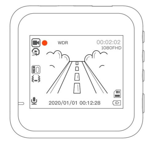
Upon starting the ignition, the camera automatically starts recording.
