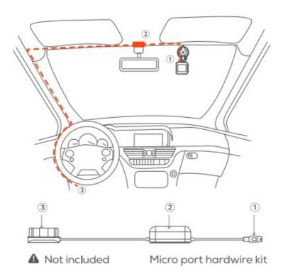
Install a Micro-port hardwire kit with the dash cam for 24/7 parking monitoring.
