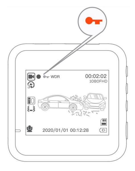
The G-sensor detects collisions automatically locks the footage as eveidence.
