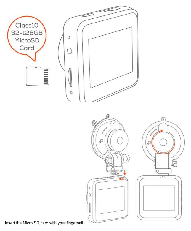
Connect the dash cam to the suction mount correctly.
