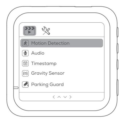
Recommended Settings: Parking guard "OFF"; Motion detection "OFF"; G-sensor "Low"; Loop recording "3 minutes";
