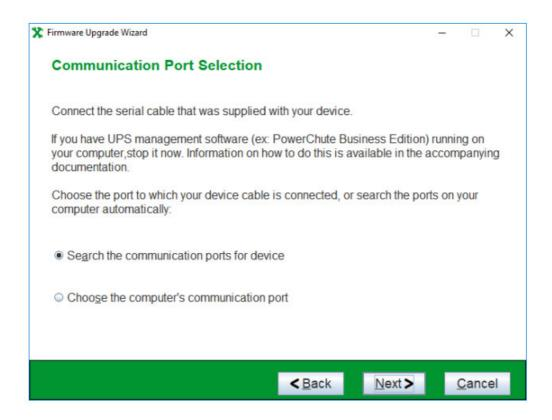
The Firmware Upgrade Wizard will now search the communication ports for the UPS. The UPS is referred to as the "device" on the screen. If you have set up virtual ports, it is important to manually select the correct port that the UPS is connected to.
