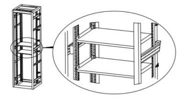
Refer to the below chart to install UPS and battery pack into 19" rack enclosure. Lift the UPS module and slide it into rack enclosure. Secure the UPS module to the rack with screws, nuts and washers (not supplied in the package) through its mounting brackets into the rails.
