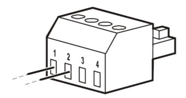
If the contacts are closed, the UPS will turn OFF and power will be removed from the load.
