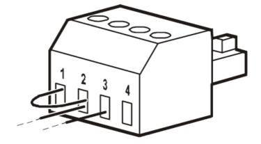
If the contacts are opened, the UPS will turn OFF and power will be removed from the load.
