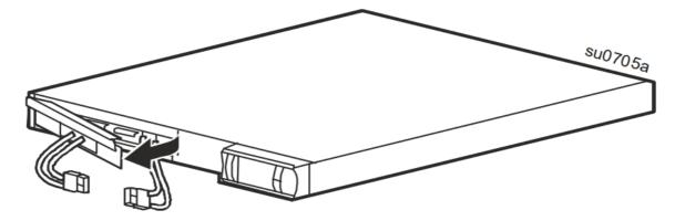
4. Slide the battery out of the UPS. Do not pull on the battery cable to remove the battery from the UPS
