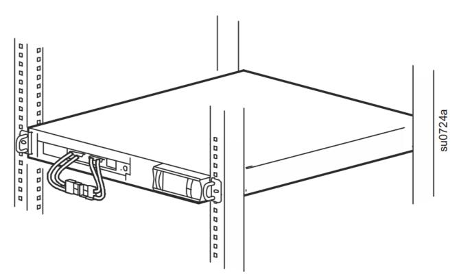
8. Install the bezel on the front of the UPS
