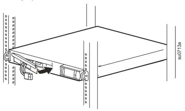
6. Secure the door with the screw previously removed
