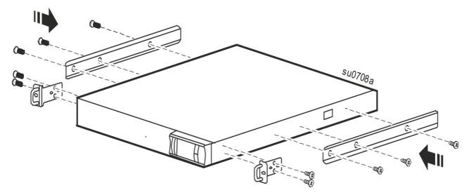
2. Install the 1U Rail Kit included with the UPS. Refer to the installation instructions provided with the rail kit.
