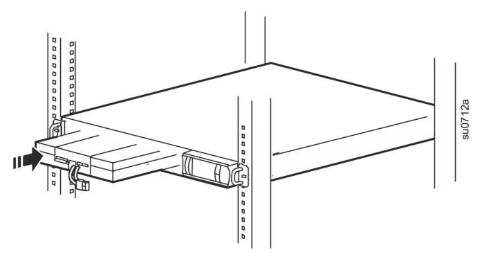
5. Install the battery compartment door
