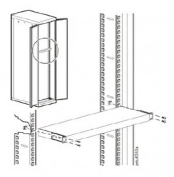
enclosure) above and below a notched hole on each vertical mounting rail in your chosen location.
