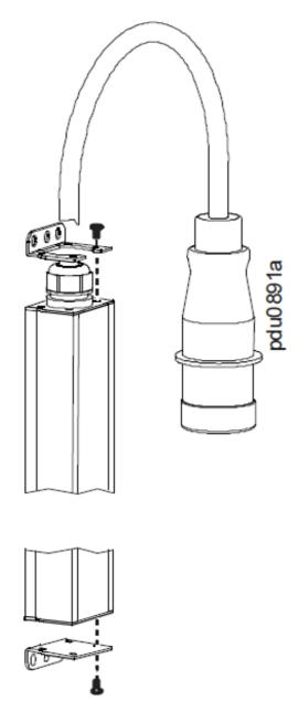
2. Install the PDU to the rack with the provided four (4) M5 x10 mm self-tapping screws.
