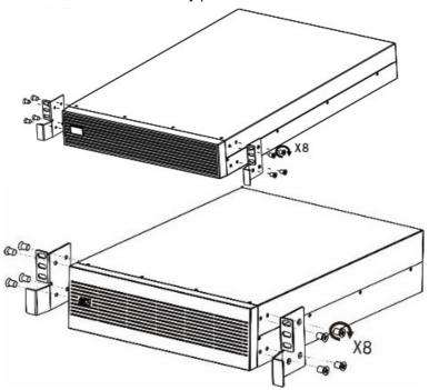
2. Lift the battery module and slide it into the rack enclosure. Secure the battery module to the rack with screws, nuts, and washers (not supplied in the package)through its mounting brackets into the rails.
