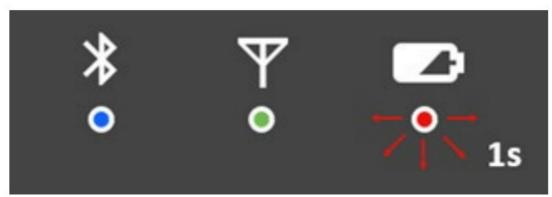
The battery level is indicated by the red LED (4) and directly proportional to the red LED light time in 1-second long cycles.
