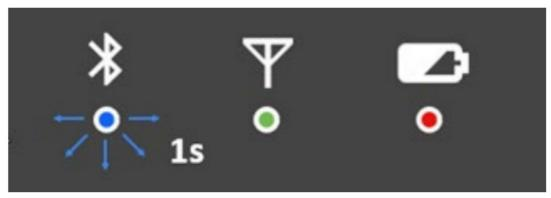
Connecting a mobile terminal to the communication module requires a standard Bluetooth pairing procedure:
