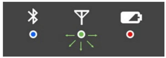
The RF receiver is active when the green LED (5) is on. Each RF data frame successfully received via Wireless M-Bus is indicated by the same LED switching off for a brief moment.
