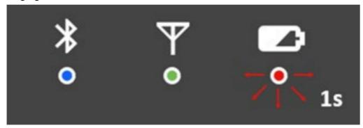
Due to the performance characteristics of lithium-ion battery packs, avoid leaving the APT-VERTI-1 communication module with the battery drained for too long. Otherwise, the battery service life will be reduced. The battery is deeply discharged when the red LED (4) blinks briefly every 10 seconds. The communication module cannot be powered on when this happens.
