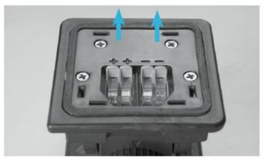
• Connect the speaker wires taking care of the polarity. Two positive and two negative connectors are supplied to allow speakers to be connected in a daisy chain system.
