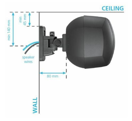
Determine the position where the ClickMount will be mounted on the wall. Please allow a minimum distance of 105 mm for MASK6C and 50 mm for MASK4C between the top of the ClickMount and the ceiling is necessary when installing the speaker in the upright position. The cable entry point is 95mm below the top of the bracket.
