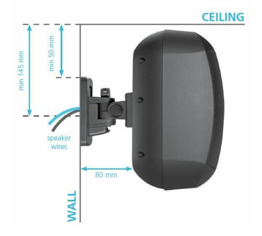
The intelligent ClickMount mounting system helps you to install the MASK4C(T) speaker in a safe and easy way. Please note the minimum distance from the ceiling and wall as shown in the drawings below:
