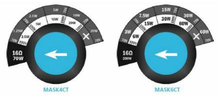
• 16 ohm position: for low impedance amplifiers only! This switch position is not compatible with 70 / 100 volt line amplifiers!
