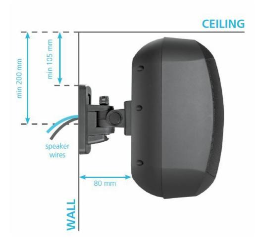
The intelligent ClickMount mounting system helps you to install the MASK6C(T) speaker in a safe and easy way. Please note the minimum distance from the ceiling and wall as shown in the drawings below:
