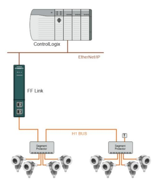
The FF Link module can connect up to 32 H1 slave devices.
