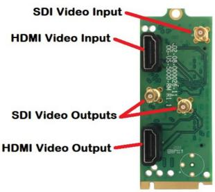
Install the Apantac OG-US-5000 rear module (RM). Secure with the included screw and washer. Insert main board in the appropriate slot to match the RM card edge connector. Insure the main board is firmly seated into the RM connector.
