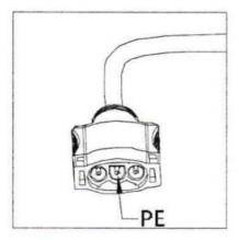
**NOTE:** Cover any unused connectors with Bus Cable Y-CONN Cap to protect the connectors.
