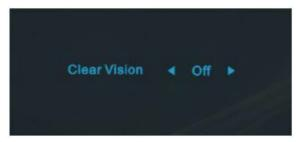
3. Press and hold "<" button for 5 seconds to activate the Clear Vision Demo, and a message of "Clear Vision Demo: on" will be display on the screen for a duration of 5 seconds. Press Menu or Exit button, the message will disappear. Press and hold "<" button for 5 seconds again, Clear Vision Demo will be off.
