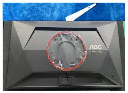
5. Remove the rear cover, then take off all of the tapes and disconnect the connectors.
