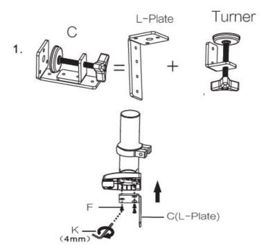
2. Once you have Secured the L-Shaped bracket to the base, attach the turner apparatus to the bracket.
