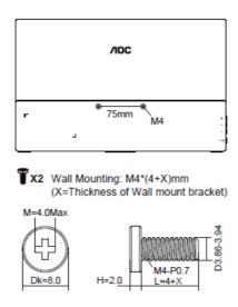
This monitor can be attached to a wall mounting arm you purchase separately. Disconnect power before this procedure.
