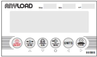
Press the [ON/OFF] button for 2 seconds. The indicator will start with self checking displaying digits 000000 to 999999. In the weighing mode, press the Zero button to return the scale to zero.
