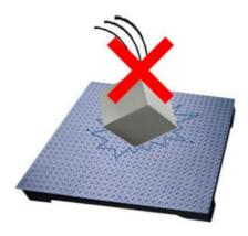
The occasional overloading may not damage the scale body but the accuracy of overloading range may not be achieved. If scale damage is caused by overloading, it shall not be covered by warranty
