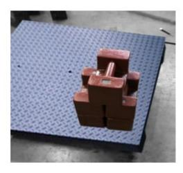
Identify which corner has the highest or lowest reading to adjust its corresponding potentiometer at the J04EA junction box. If lowest reading is selected, adjust its corresponding potentiometer clockwise to increase its reading making closer to the reading of at the center. Or,
