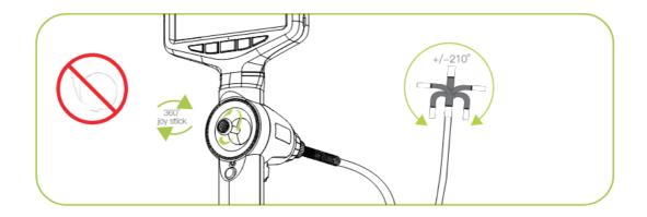
A Tips: To achieve the max articulation angle, the cable should not be coiled in a circle.
