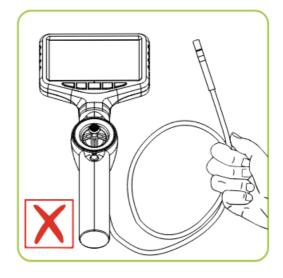
Notice When using the borescope, it is important to emphasize that the coil should not be wound up as this can affect the steering function and cause the articulation angle to become smaller.
