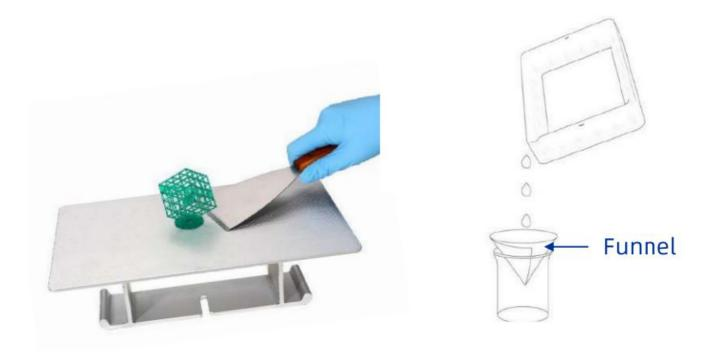
[IMPORTANT] Inevitably, in case of incomplete curing or failed prints, there might be some cured resin left in the vat. It is suggested to filter the resin by a funnel and then store the liquid in a sealed container. The residues left on the platform or in the vat can be wiped off with paper towel.
