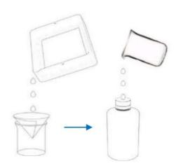
(4) Do not left resin in resin vat for over two days when it is unused. Please filter and store the resin properly.
