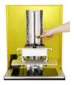
(1) If Z axis make noisy sound, please apply lubricant to z lead screw.
