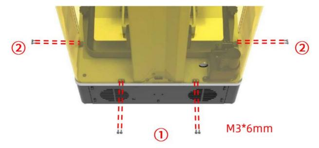
12. Turn the machine back and install resin-holding bracket first.
