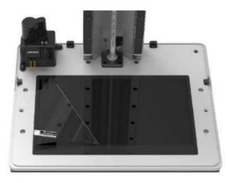
4. Loosen the four screws on the printing platform.
