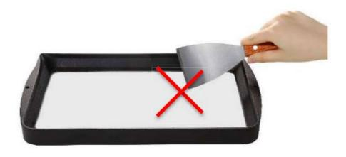
(2) Clean off the residues cured on FEP film when the printing fail: Set full-screen exposure for 20s and then remove the cured resin sheet to protect the film. Do not use sharp objects to scrape off the residues on FEP film.
