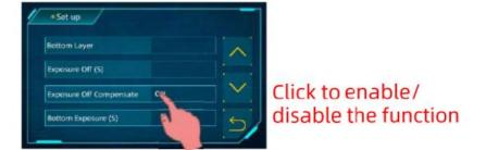
The compensation only works on bottom layers and layers with large area. In normal layers, off time is automatically added according to the area of layers; the larger the area, the longer the off time.
