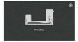
3. When the printing fails, resin may be cured partially in the vat. Please set to Vat Cleaning and remove the residue. Otherwise, it may cause damage to the release film or LCD screen.
