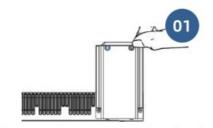
Loosen 2 screws on the back
