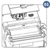
Put resin vat with its feet stuck in locating holes
