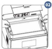
Tighten the two knobs
