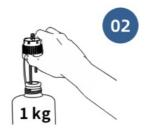
Insert the cap part to the resin bottle and tighten it
