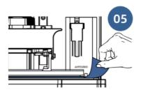
When pulling the leveling paper, there is a significant resistance or it cannot be pulled out
