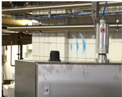
From Bolt to Bolt. An Anybus Wireless Bolt is mounted on the top of the baking machine (left) and communicates via Bluetooth to another Wireless Bolt on the top of the controlling cabinet (right). communicates via Bluetooth to another Wireless Bolt on the top of the controlling cabinet (right).
