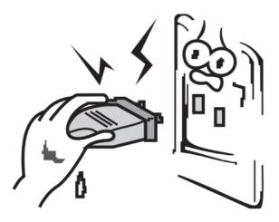
Do not use a broken power plug nor keep power cord near heat source; otherwise, electric shock or fire may occur.
