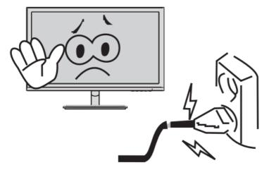
When cleaning the device, be sure to remove the power plug, use a piece of soft cloth rather than industrial chemical to clean the device, be sure not to let water enter the device.
