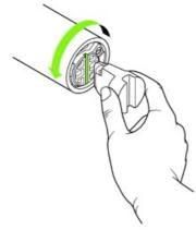
3. The 18650 battery will slide out with the negative side facing outward.
