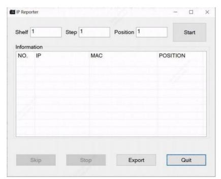
7. On the controller board, click the IP Report button. Hold it down until it beeps (about 5 seconds). The IP address will be displayed in a window on your computer screen.
