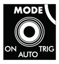
When in this position, the amplifier is always on.
