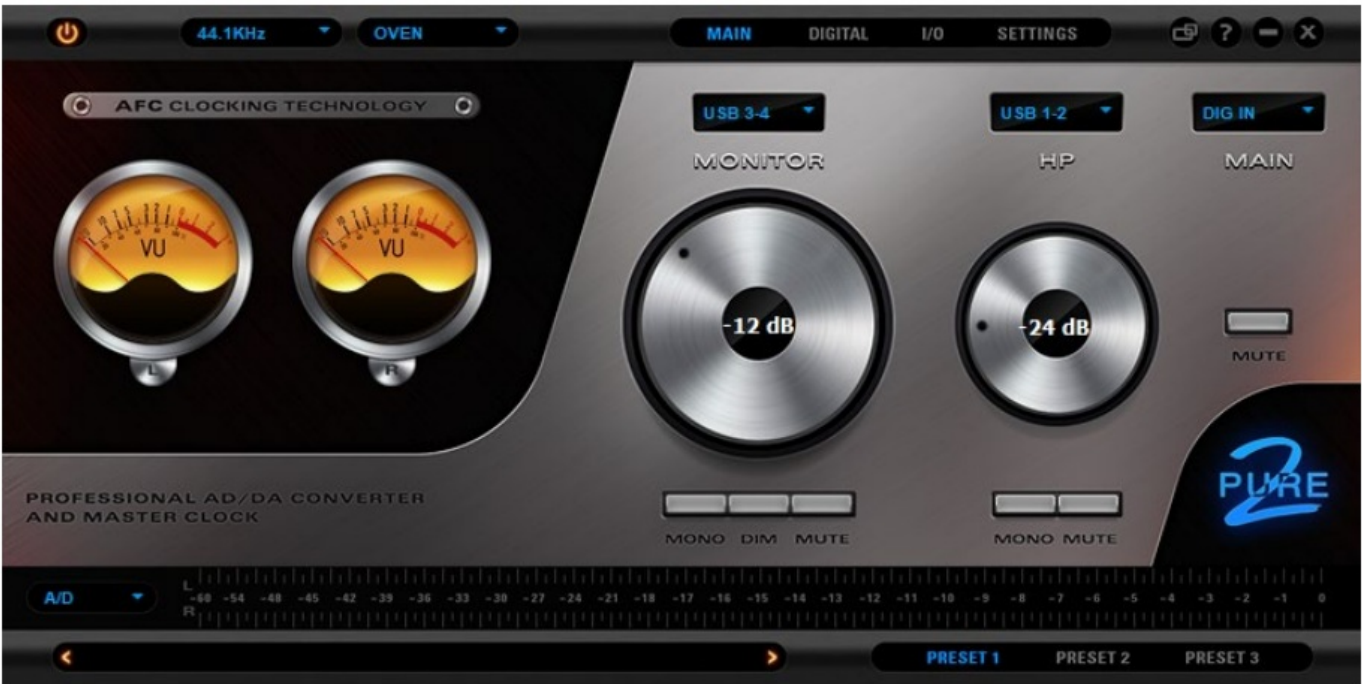
Features Monitor and Headphone audio source selectors, volume rotary controls and buttons – ‘Mono’, ‘Dim’, ‘Mute’.
