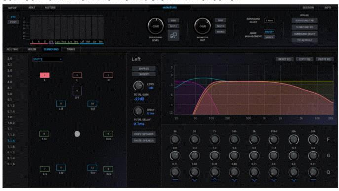
The Antelope Audio Surround / Immersive Monitoring System provides monitoring control functionality and speaker calibration processing for up to 16 channels of surround or immersive audio. Formats from stereo up to 9.1.6 Dolby Atmos are supported while maintaining customizability within the 16-channel limit for any unorthodox setup requirements.
