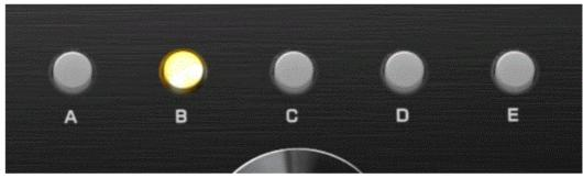
Presets A-E buttons allow for fast Software Preset recall buttons for all of the interfaces' settings, including signal routing, audio format switching, output levels, and speaker calibration. They can be configured in the Session tab of your interface's control panel, as follows.
