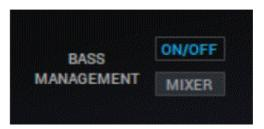
Mirrors the Control Panel Bass Management On/Off Switch. Useful for checking between having the LFE channel play all low-frequency contents of the mix or only its designated signal.
