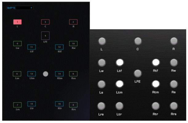
Selected multichannel formats are represented here. Buttons on the MRC will become inactive when their respective speakers are not part of the selected format.
