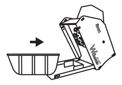
The fluid tank is designed to fit only one way around. Make sure you insert it correctly, as shown above, with the lower edge facing into the machine.
