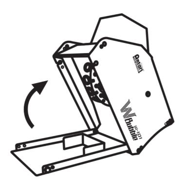
Once the screws are removed, the lid of the housing can be carefully swung upwards, as shown above. Take care not to spill any of the bubble fluid inside the unit.
