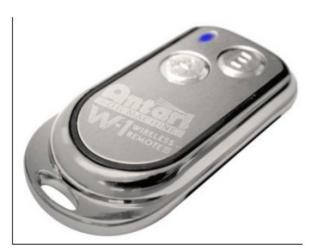
With the transmitter, it is possible to output via radio over a distance of up to 50 meters. The transmitter is compatible to any receiver of SW-250 and can control an unlimited number of machines in parallel. Press the button "A", to output. As a control, the LED on the transmitter is lit. To stop the output, press the button "B".
