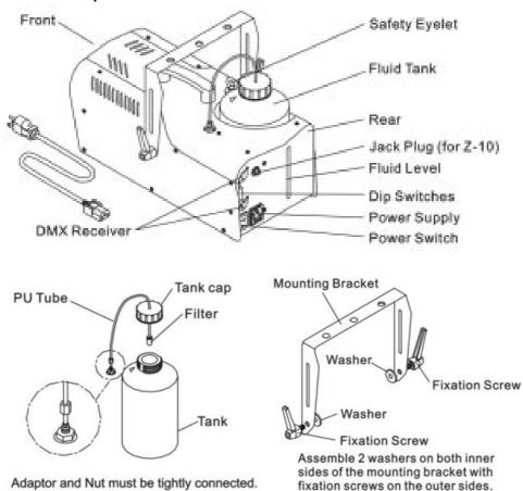
Note: A fluid level sensor is installed on the unit. The machine will stop to fog if the fluid is lower than usable level.
