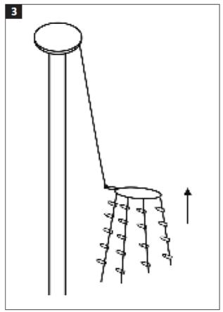
3. Fasten the product to the ground around the flagpole. Make sure all the parts of the product are evenly spaced to each other and the flagpole. Roll up surplus string light on the bobbins.
