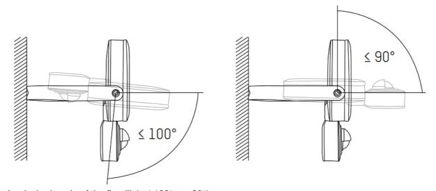
• Set the desired angle of the floodlight  $(-100^{\circ} \text{ to } +90^{\circ})$ .
