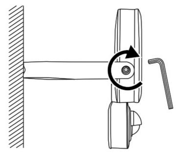
• Tighten the set screws with a hex key.
