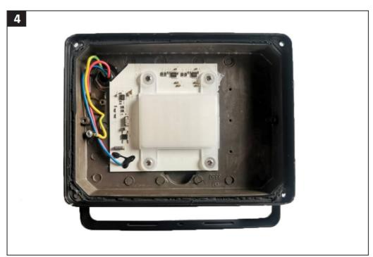
4. Cut the wires and remove the LED module.
