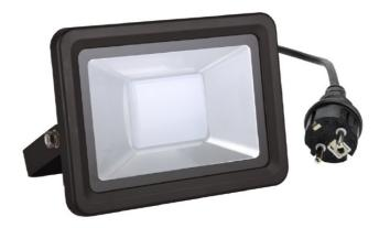
The glass is glued on the casing for 30 W and 50 W. To remove the glass, put tape on the glass to protect it if it breaks and warm with a hair dryer to soften the glue. Carefully remove the glass with a knife. Remove the reflector.
