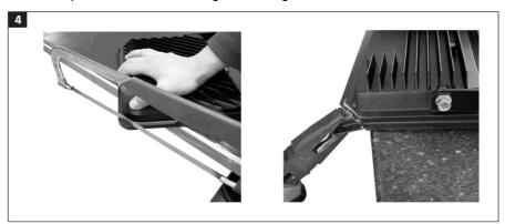
3. Insert a flat-tip screwdriver in the gap between the glass and the casing, and carefully pry both parts apart.
