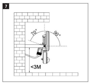
2. The detector can be turned  $70^{\circ}$  to the right and left, and up  $90^{\circ}$  and down  $80^{\circ}$ . FIG. 8
